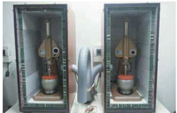
Panels added to existing box to enhance quietness.
